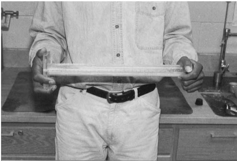
**Figure 4**—Using Hand Method of Shaking
