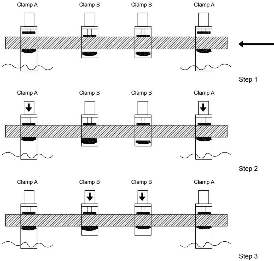
**Figure 3**—Specimen Clamping Procedure
