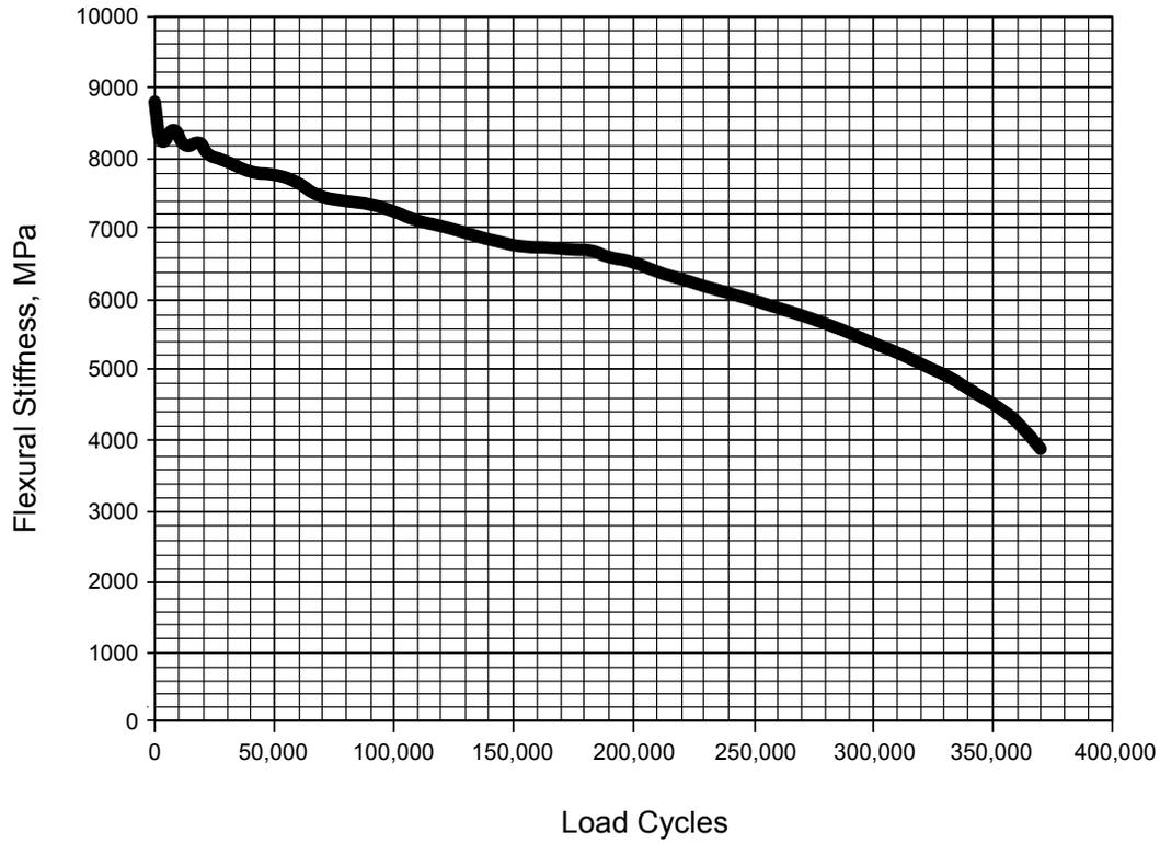
Figure 6—Stiffness versus Load Cycles
