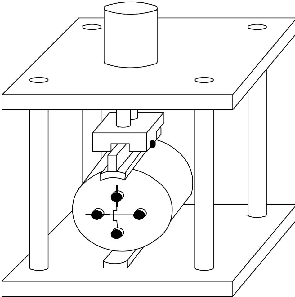
**Figure 2**—Specimen Loading Frame
