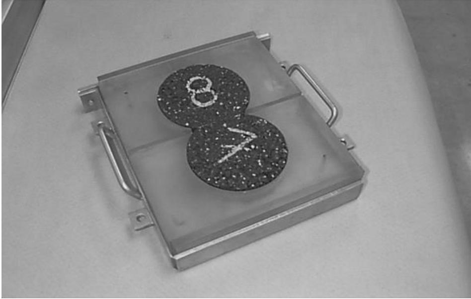
Figure 1—Cylindrical Specimen Mounting System
