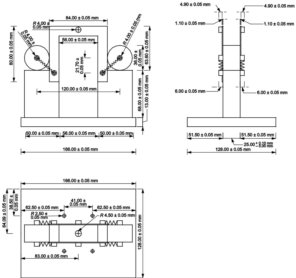
**Figure 2**—SCB Test Fixture
