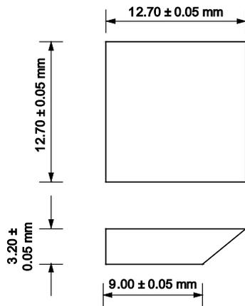
**Figure 4**—CMOD Gauge Knife Edges
