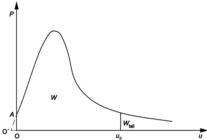
**Figure 7**—Load versus Average Load Line Displacement ( $P - u$ ) Curve
