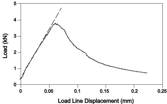
**Figure 8**—Example of Stiffness Determination
