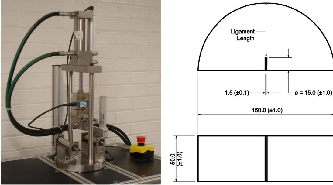
**Figure 1**—SCB Test Specimen and Configuration (dimensions in millimeters)
