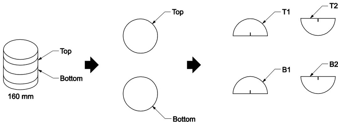
**Figure 3**—Specimen preparation from SGC specimens
