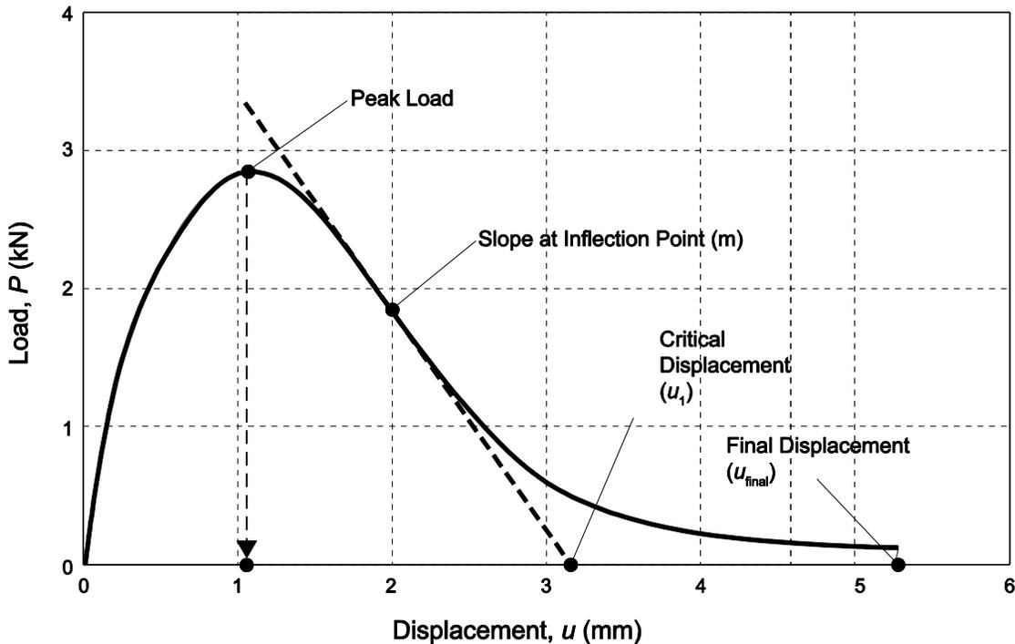
**Figure 4**—Recorded load ( $P$ ) versus LLD ( $u$ ) curve
